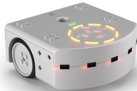
Fig. 1: The Thymio II robot (110x112x54mm).
